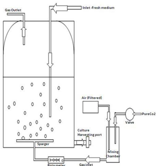
Figure 1: Schematic diagram of lab scale 2L Photo bioreactor
